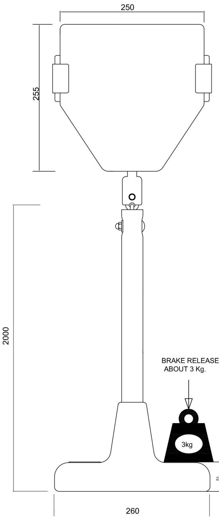
**GB** -When the R&T pendulum seat is connected to the R&T cableway trolley – the user must apply a weight load/force of approximately 3,0 kg to the pendulum seat in order to release the brake in the trolley.
